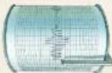
Vibrations are recorded by a pen on a paper trace rolled over a drum.
